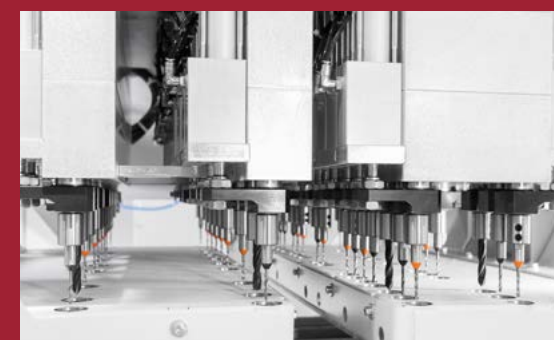
Special drilling head for vertical drilling
