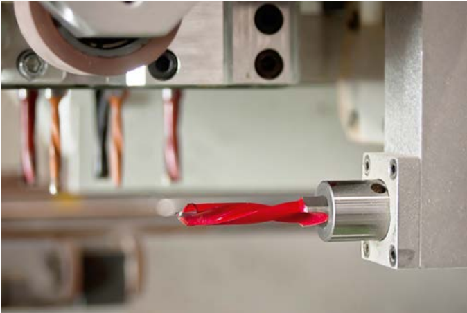
Long edge-drilling unit
