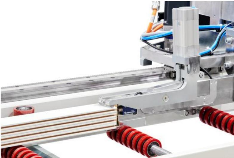
A clamping claw clamps the workpiece or package and moves it to the trim saw.
